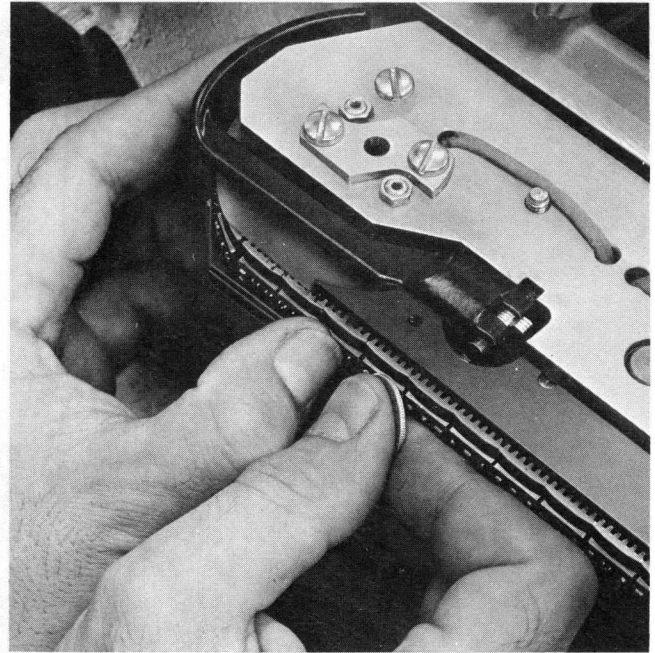
Figure 4-44. Method of Separating Type Slugs
