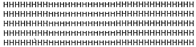
Figure 1-43. Light or Missing Tops
