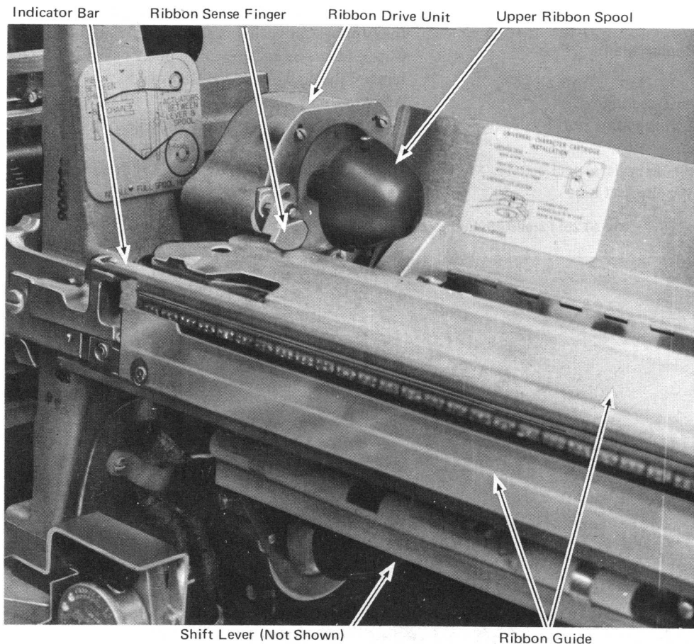
Figure 4-54. Ribbon Drive Assembly
